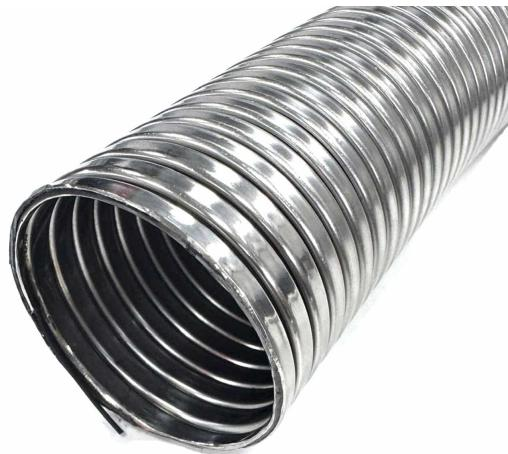
Stainless steel Rubber packed Interlock combines the mechanical strength and flexibility of stripwound metal tubing with enhanced air-tightness provided by a rubber packing between the interlocked metal profile. This product delivers a combination of flexibility, durability, and improved sealing.
